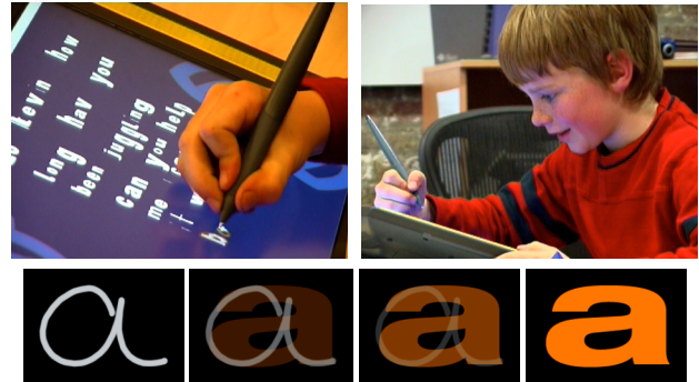
Figure 3: Polymorphic Letters affords a more fluid and personal writing technology. The idiosyncratic attributes of your hand lettering such as size of the letters and pressure of the pen on the tablet are translated into colourful typographic forms. The transformations, visualised by means of a blend, will eventually include a range of imagery and sounds.
